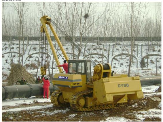
GY90 full hydraulic sideboom is developed by our own technology. It has full hydraulic driving, micro computer control and specialized chassis. Our GY 90 full hydraulic sideboom adopts harmonious uniform of machine, electric, and hydraulic mechanisms with advanced control system. It has many advantages, they are high automation degree, smooth traveling, simple operation, high efficiency & energy saving, safe & reliable and low maintenance cost.
